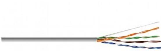
Kramer's BCLS-11 is a high-performance CAT 5E U/UTP cable designed for IT, LAN and Ethernet installations. BCLS-11 is constructed with four pairs of 24AWG solid bare copper conductors in an LSZH jacket with internal rip cord and sequential markings every meter. It is packed in a Reelex II carton for easy to pull-out. BCLS-11 exceeds CAT 5E specifications to provide additional performance and bandwidth beyond the basic standard
